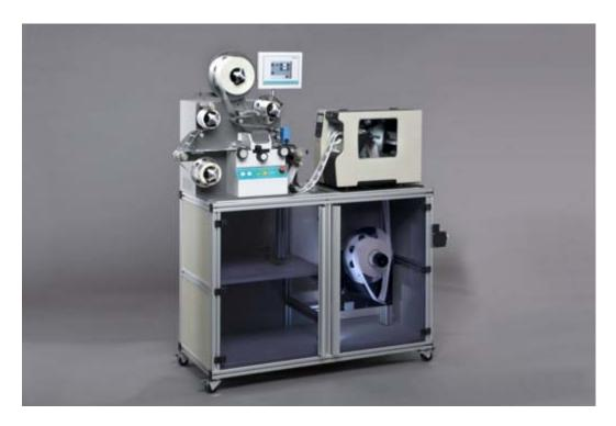
There the label is cut using a customized die, cookie-cutter style, and laminated via cold-press, all in one step. The finished labels, are then rewound on a take-up spindle while the waste matrix is stripped (removed) and rewound on another spindle for later disposal. Voila - beautiful, custom labels with a consistent, virtually impregnable matte or glossy laminate covering. The possibilities are endless.
